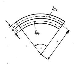
If the length of the strip at temperature t=0°C is  $l_0$  then at temperature t=400°C the copper strip will have the length
