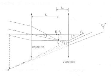
A telescope is used to magnify objects that are very far away; in most cases the object can be considered to be at infinity. The astronomical telescope contains two converging lenses located at opposite ends of a long tube. The lens closest to the object is called the objective lens and forms a real image  $I_1$  of the object at its focal point  $F_0$ (or near it if the object is not infinity). Although this
