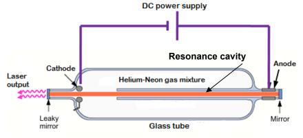
The photons moving parallel to the tube axis are still moving to and fro due to reflections from mirrors. A chain reaction builds up rapidly in this direction accounting for the inherent parallelism of the laser light.
