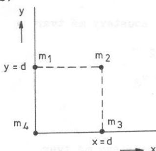
$$x_o = \frac{\sum_{i=1}^4 x_i m_i}{\sum_{i=1}^4 m_i} = \frac{x_2 m_2 + x_3 m_3}{\sum_{i=1}^4 m_i} = \frac{2d + 3d}{10} = \frac{d}{2} = 5 \text{ cm}$$
